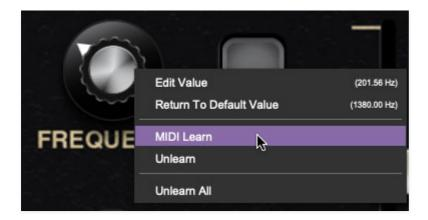
Begin by right-clicking on the *Frequency* knob in the VCF section and selecting *MIDI Learn*. A transparent purple overlay appears over the entire slider indicating that it's in learn mode. Now move the desired hardware control device. The purple overlay disappears and the hardware control will move the onscreen knob. If you get cold feet (or accidentally put the wrong control into learn mode), learn mode can be aborted by right-clicking and selecting *Stop Learning*.
