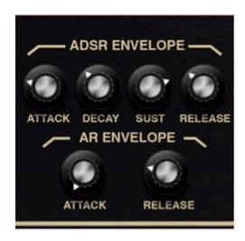
Pro-Soloist includes two envelope generators - a standard ADSR (attack/decay/sustain/release), and an AR (attack/release). These are most often used to modulate the VCA for shaping the amplitudes of notes, but also can modulate a number of other destinations using the cream-colored sliders and the Mod Matrix.
