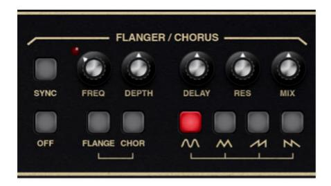
We've included a thick and warm flanger/chorus effect. Flanging and Chorus are closely related - the general difference being that flangers use a shorter time range and some amount of feedback (this intensifies the "jet-flyby" whoosh), whereas choruses utilize a slightly longer delay time, and no feedback.
