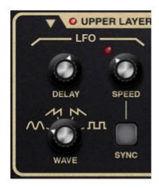
The LFO (low-frequency oscillator ) generates sub-audio range signals intended for modulation purposes.
