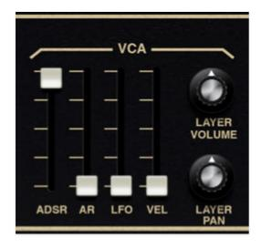
VCA is short for "voltage-controlled amplifier," and for all intents and purposes, you can think of it as the automated volume knob the controls the amplitude of each note played. It has a number of mod sources, but is primarily controlled by either the ADSR or AR envelope generator.
