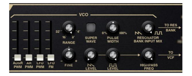
VCO is short for "voltage-controlled oscillator." There's just one oscillator per voice, but the Pro Soloist's unique architecture gets a heck of a lot of mileage out of it. Here's the rundown of its controls:
